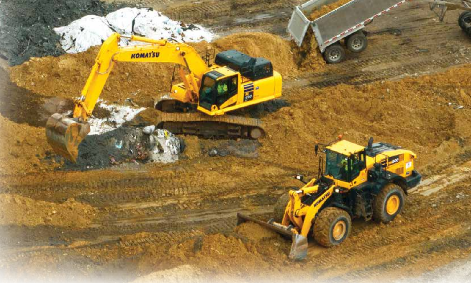
Operators work in tandem to move material with a Komatsu PC490LC-11 excavator and a WA500 wheel loader at the Republic Services Cedar Trail Landfill.
